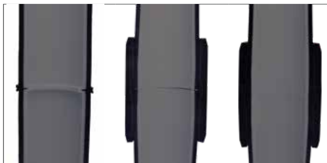
Heated element butt welding
